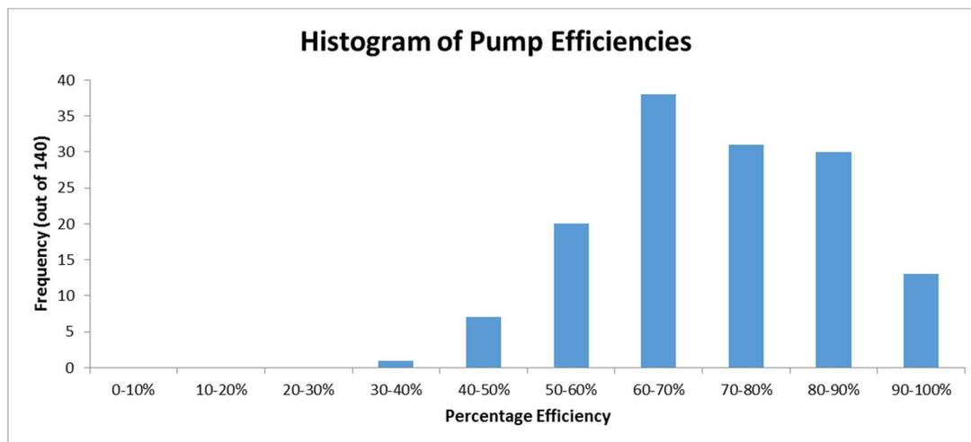
The information shows that there were 8 pumps with efficiencies less than 50% and 13 pumps with efficiencies more than 90%. The rest of the 140 pumps have efficiencies between 50% and 90%. An efficiency of 50% means that the pump use twice as much electricity as it should.
