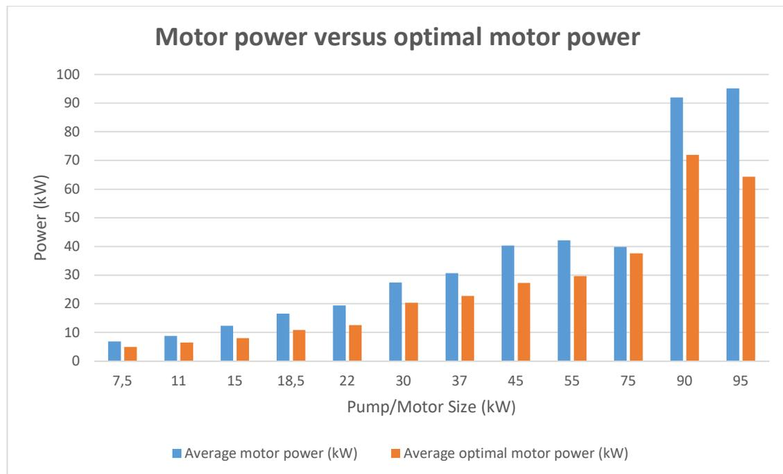
The optimum power is obtained from a PSAT computer program which is in line with the relevant manufacturer pump curve information. The information shows that the actual power consumed was more than the optimum power for that pump. On average the pumps consume 39% more power than what is considered optimal. This means that a 28% saving from current values is possible. The next graph shows a histogram of the pump efficiencies for the same sample of 140 pumps.
